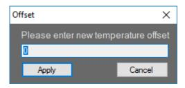
Offset values are stored inside the EEPROM and are therefore unique to the device and transferred to all systems that you use this particular device on.
