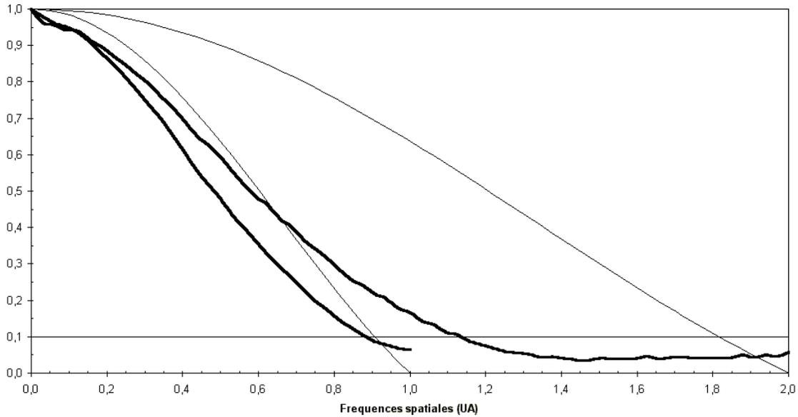
In this operational mode the camera resolution never attains the theoretical value, even with the B&W chip. The resolution in 640x480 is only 1.3 times better than the 320x 240 mode. The main advantage, and it is a significant one, of the B&W adaptation is the threefold increase in sensitivity.
