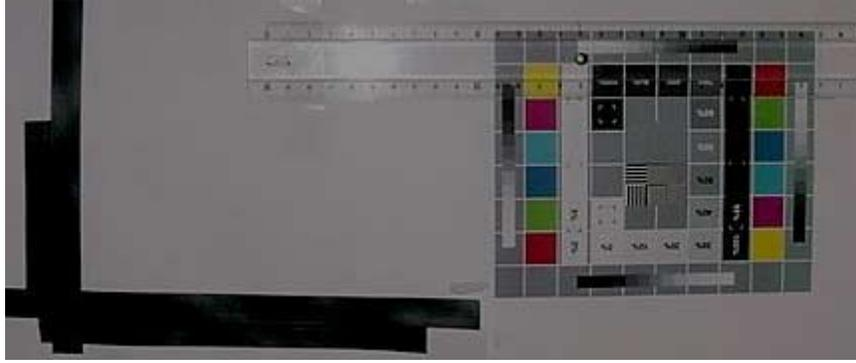
The exposures were performed using PRISM 5.0 at a rate of 5 frames per sec., and one unique BMP image was recorded. The camera settings were: contrast 100%, gamma 0%, saturation 100%, brightness about 40% in order to avoid saturating the whites, and white balance was set to automatic. As well, the enhancement of the vertical contrast and the reduction of “noise” to zero were assured by the Setwc software.
