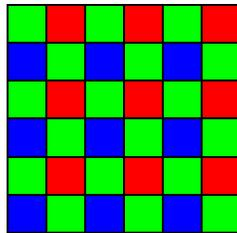
To produce a colour image (RGB 640x480) with this matrix the internal software of the camera performs a certain number of calculations. The different RGB values of the colour image are given as the average of the neighbouring pixels :
