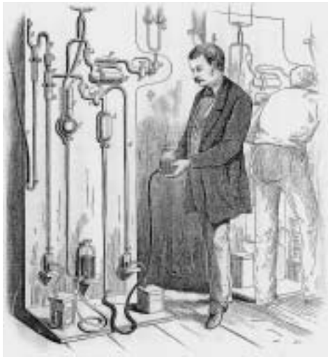
Figure 2. Vacuum pumping, 1880s style. This type of vacuum pumping system was used by T. Edison in the early manufacture of light bulbs.
