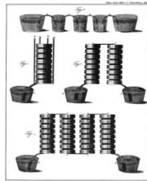
Figure 3. Four connections of “voltaic piles” (alternate silver and zinc discs separated by moist paper) as described in A. Volta’s letter to Sir Joseph Banks of the Royal Society of London bearing the title “On the Electricity excited by the mere Contact of conducting Substances of different kinds,” dated March 20, 1800.
