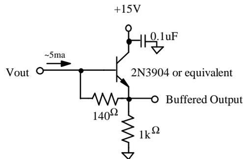
Figure 4 - Recommended Output Structure Load Diagram
