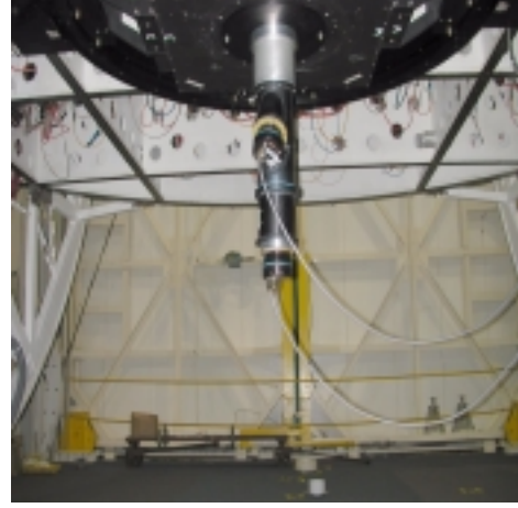
Figure 10: The interferometric Hartmann wavefront sensor attached to the f/9 top box of the 6.5m MMT. Using the instrument rotator, the Hartmann apertures of the wavefront analyser were carefully aligned with the axes of the primary mirror support system.
