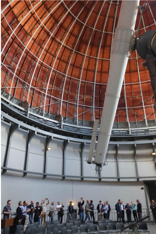
Figure: Workshop participants viewing the 77-cm refractor of the Nice Observatory, which dates from 1886. The dome was designed by Gustave Eiffel, architect of the famous tower. (Picture by Matic Smrekar.)
