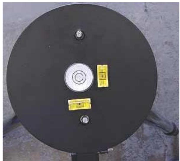
Note: The side where the bubble stays is the side that should be lowered.
