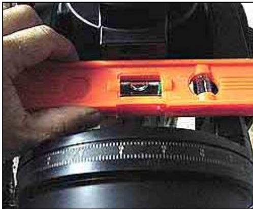
Press the bubble level against the attachment pad to eliminate the front and back effect.
