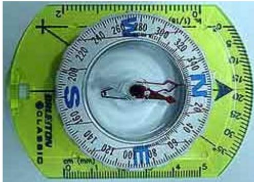
The compass must have a “declination scale” which you can adjust. A high degree of accuracy is not expected from using a magnetic compass for alignment. This is to be used only when Polaris is not visible.
