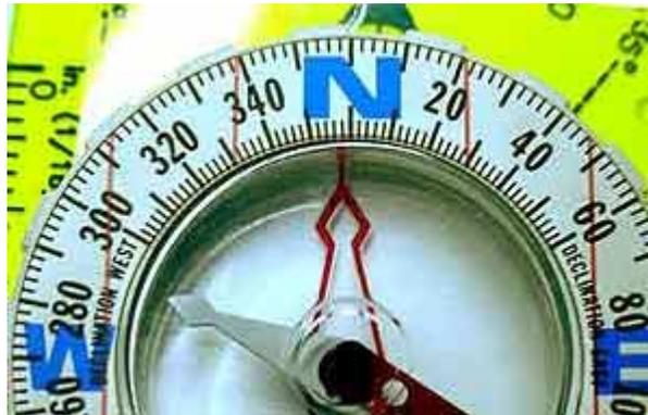
Note: Eastern magnetic declination is to the right of the "North" position and western magnetic declination is left of the "North" position. As an example, Figure 22 shows the correct setting for 16° West declination, which covers Providence, Rhode Island.
