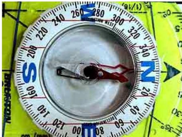
Note: You can turn the declination dial at the correct declination value to align it with the centerline of the compass base and turn the telescope until the needle point to the N mark on the compass.
