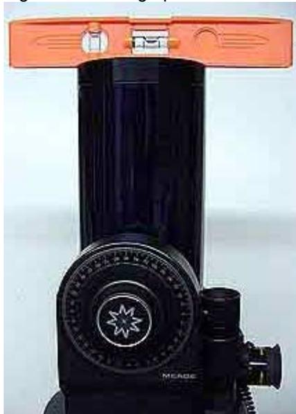
Long bubble level resting on top of the lens.
