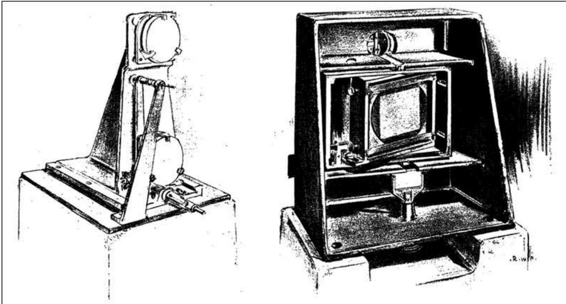
Figure 15- Concave mirrors of the spectrohelioscope (left) and grating support and line-shifter.
