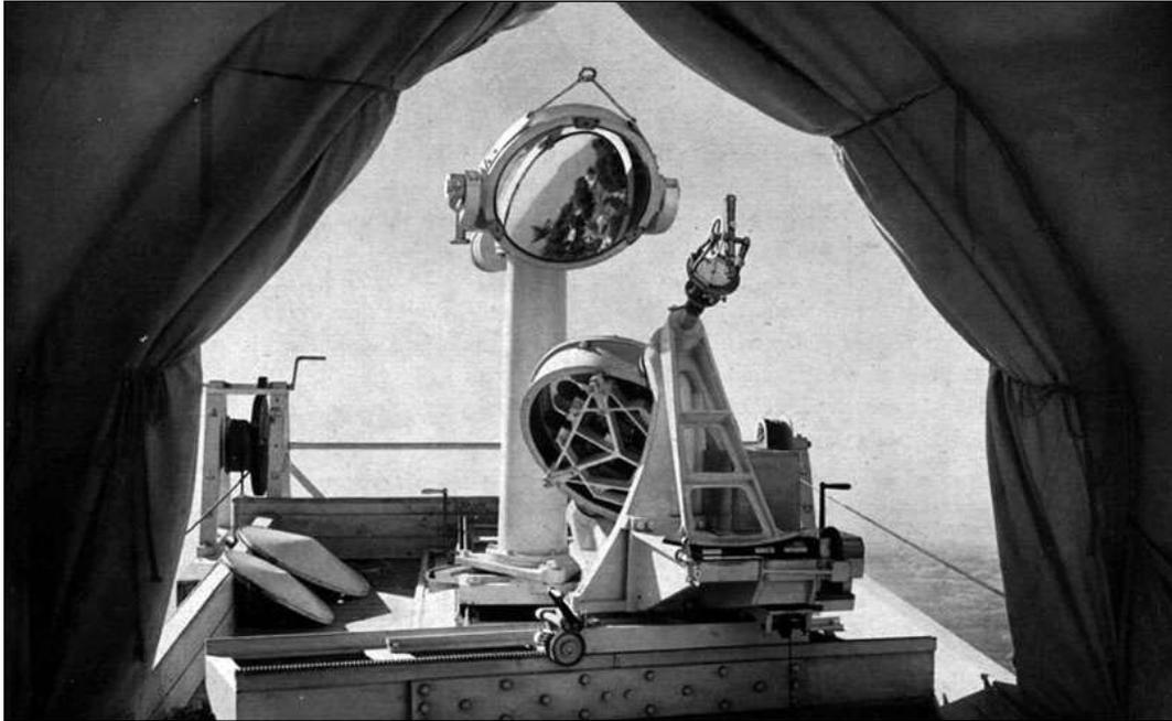
Figure 7- Coelostat of the Snow horizontal telescope.
