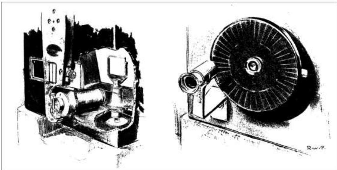
Figure 16- Second slit, driving mechanism, line-shifter (left) and spinning disk with radial slits (right).
