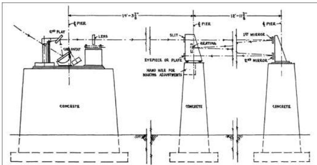
Figure 12- Concrete piers for the coelostat and spectroheliograph.
